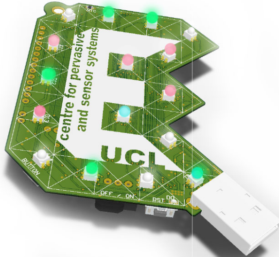
Figure 2: 16 Red, Green, Blue LEDs on one side of the board
