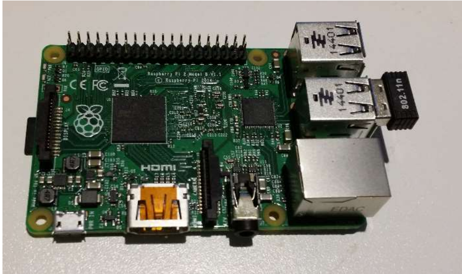
Figure PI-1: A Raspberry Pi 2, with the USB Wi-Fi module attached on.
