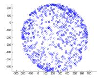
This isn't quite a circle but it's fairly close (there is some distortion or the sensor is slightly wonky). What we would like to do is to move the centre of the circle to (0, 0), so that if you hold the Engduino flat, we can work out which direction you're facing in. One simple way of estimating the
